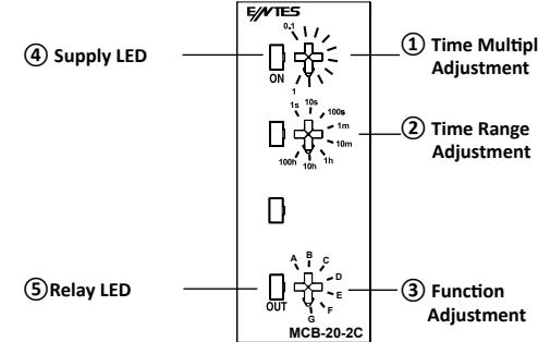
**① Time Multiplier Adjustment:** It is the time multiplier that the selected time range is multiplied. It is set from 0.1 to 1 with the adjustment trimpot on the device.
